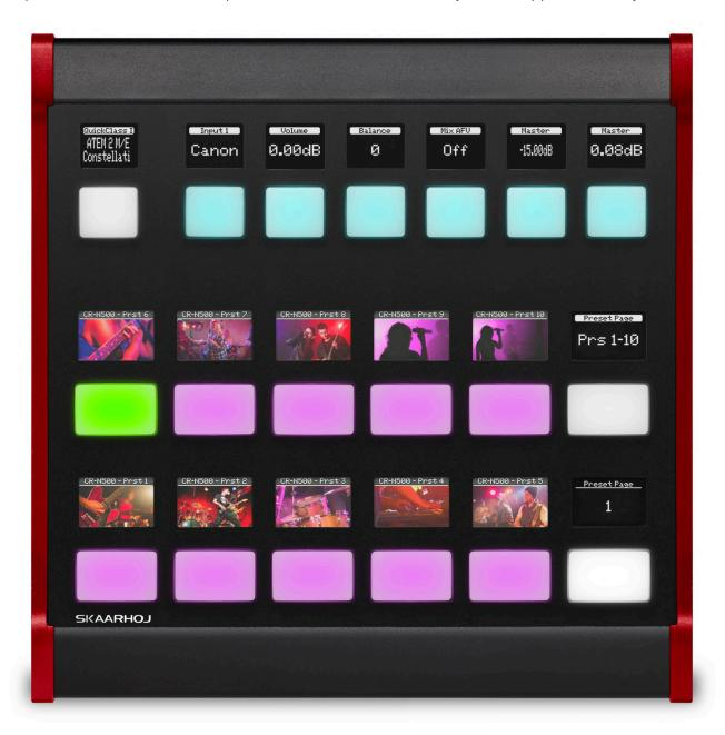
The Frame Shot Pro also features seven customizable four-way buttons that increase functionality and can be configured for various actions. When used with the RC-SK5 Pro License, these buttons gain even greater versatility through Quick Classes, which offer ready-to-use configurations for a wide array of devices, including video switchers, routers, and audio equipment.
